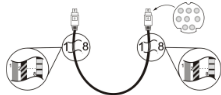
Figure 5: Straight-through 1-to-1 mini-DIN8 cable
