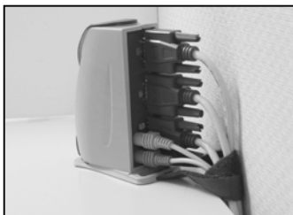
Figure 4: Velcro ties the cable sets and extends the base of the SOHOTower .
